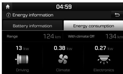
Current electricity use for drive train, climate and electronics parts are displayed. The current reachable range when Range and Climate are turned off is displayed.
